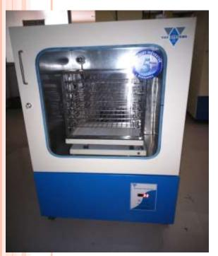
**PROVIDES AN IDEAL STORING ENVIRONMENT FOR THE PLATELETS. THIS UNIT DESIGNED TO MAINTAIN A STABLE AND UNIFORM** TEMPERATURE OF 22.0°C, THE **USER-FRIENDLY DESIGN INCLUDES AN ACRYLIC INNER** DOOR, AND SEE THROUGH OUTER DOOR, SIMPLE CALIBRATION IS **POSSIBLE VIA THE CONTROL** PANEL. THIS, COUPLED WITH A VISUAL AND AUDIBLE ALARM SYSTEM, ENSURES THAT YOUR SAMPLES ARE BOTH SAFE AND SECURE, BUT ALSO EASY TO **ACCESS WHEN YOU NEED THEM**
